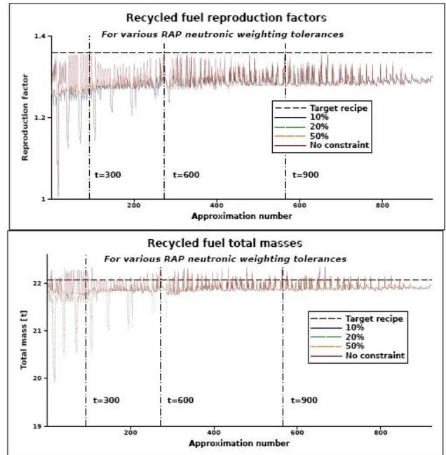
Fig. 2. Effects of neutronics constraint on neutronics and total mass performance of achieved recipes. of constraints and objective functions.
