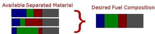
Fig. 1. Matching spent fuel from three waste streams into one MOX fuel recipe. Note: The different sections represent various isotopes within the respective barrels.
