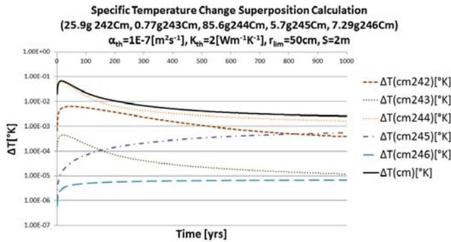
Fig. 2: As a demonstration of the calculation procedure, scaled temperature change curves for five curium isotopes are super imposed to achieve a total temperature change (note log scale).
