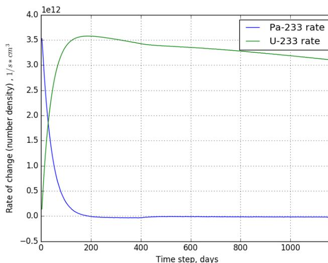
Fig. 5: Materials flows rates for the protactinium decay tank during MSBR online reprocessing.
