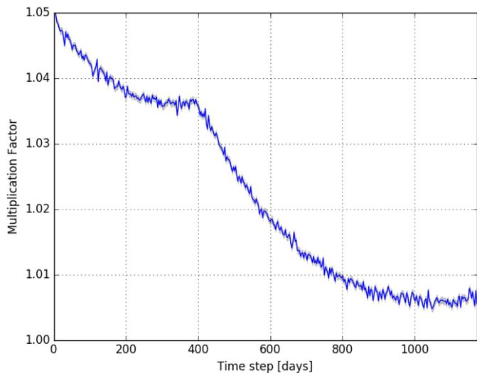
Fig. 2: Infinite multiplication factor during a 1200 days depletion simulation. The confidence interval  $\pm\sigma$  is shaded.
