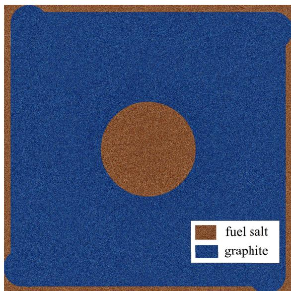
Fig. 1: Molten Salt Breeder Reactor (MSBR) unit cell of Zone I geometry.
