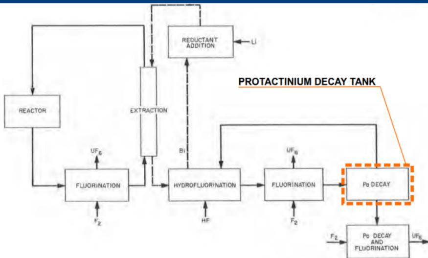
Figure 7: Protactinium isolation with uranium removal by fluorination [3].
