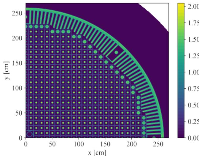
Figure 12:  $^{232}\text{Th}$  neutron capture reaction rate normalized by total flux
