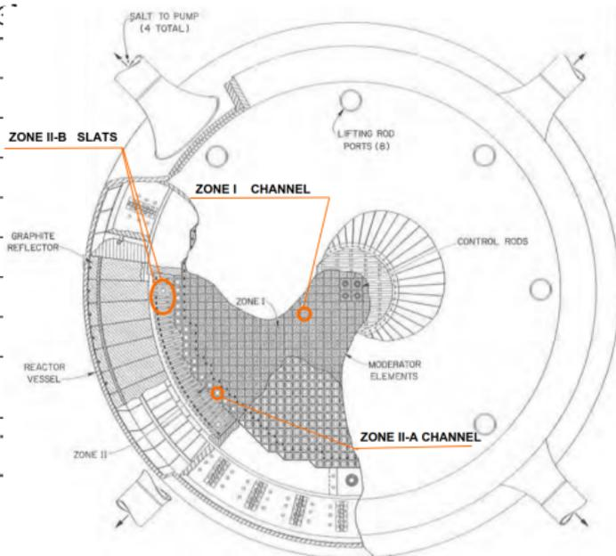
**Figure 2:** Plan view of MSBR vessel [3].
